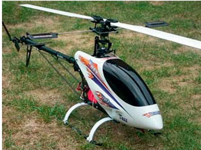
Abb. 2.3-1 Model-Helicopter T-REX 600 frame without motor and accumulator
