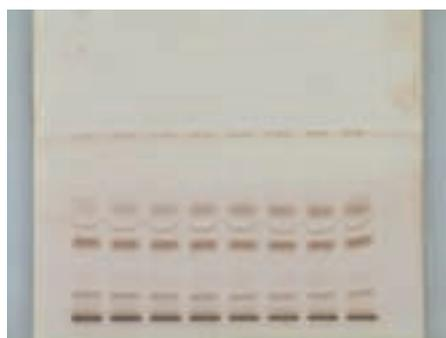
**Fig. 3.5-3:** shows eight melamine spiked milk samples (each with 1  $\mu$ L applied), stained with starch/iodine reagent
